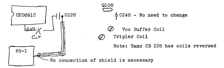
No need to adjust tripler coil, it works just fine.
