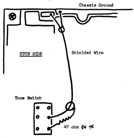
NOTE: Switch is viewed looking down on chassis from etch side.
