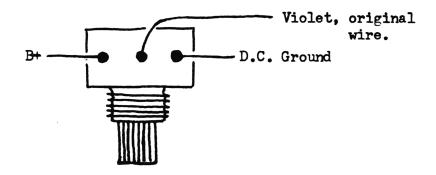
Above configuration gave approximately +6KHz after centering and realignment.
