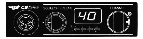
Had someone send all of the FOX units to me for evaluation. The Mdl. 240 is a very compact unit - actual size is above: S/N: 0006574, out of the box.... 3W, 35% modulation.
