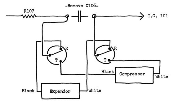
Wire the relay up as shown above, keying line below:
