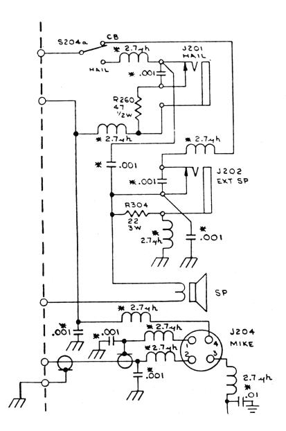
Above diagram shows revision to mike and speaker circuit for the Horizon 29A. Check against your original schematic or SAMS.
