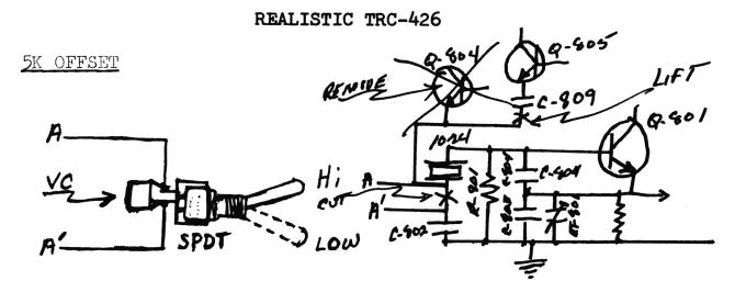
NOTE: This is a phone type unit. The best place to mount the switches would be on the back chassis wall. Drill the holes at the point where the two clam shell covers meet.
