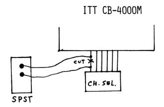
Cut #1 wire as shown and add switch. This gives Channels 41-59.
