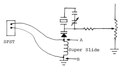
This method didn't work due to lead lenght. We overcame this by using a transistor for switching, located next to the Super Slide as shown here:
