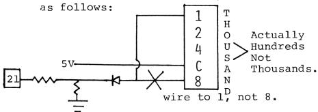
Also, the method of channel entry is in a code from 000-199 as shown on page 34 of Vol 6. You can't dial in "785" for 27.785. Rather, you must dial in "173" as per chart. The Tens, Hundreds, Thousands should really be Ones, Tens, Hundreds. Note: The thousands switch could be a simple SPST switch instead of the more expensive thumbwell type.
