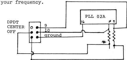
The following can be done if you would like to be able to switch over to even channels, such as 26.750. Add a 10micro-henry choke and adjust trimmer to adjust for on-frequency operation. Switch to 0's or 5's with a SPST switch.
