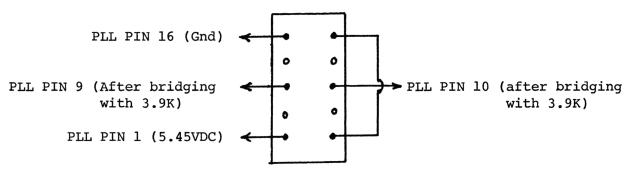
With this configuration the Delta Tune Switch selects frequency mode:
