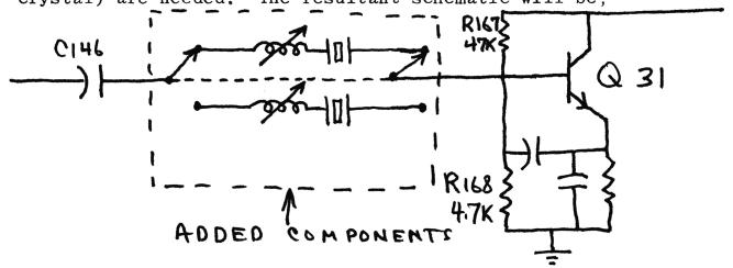
The circuit board should include the two crystals and two coils. The coil-crystal combinations are wired to the throws of the PC-CB switch. The wipers of the switch should be wired to the original Y2 mounting holes in the 8092 circuit board. The added circuit board should be installed as close to the PA-CB as possible and with wire as short as possible to minimize frequency variations caused by stray inductance.
