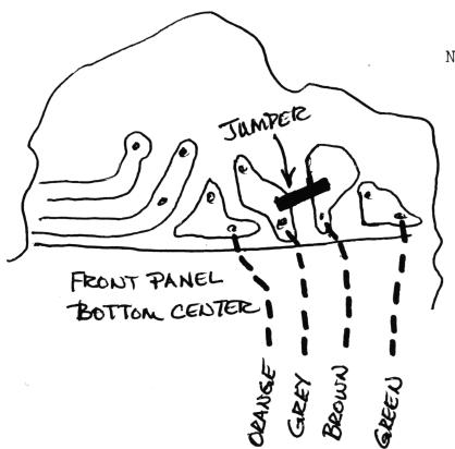
NOTE: To use the channels properly, see the chart on the next page. Unit may not receive above channel 11 on some units because of extreme frequency coverage.
