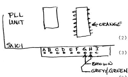
(1) Remove unit from case and unsolder the four wires from the Delta tune switch to the four connections on the front edge of the PC board, as shown.
