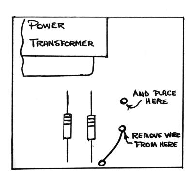
NOTE: This modification will result in 20KC coverage of the fine tune control and a power output on SSB of about 20 watts.
