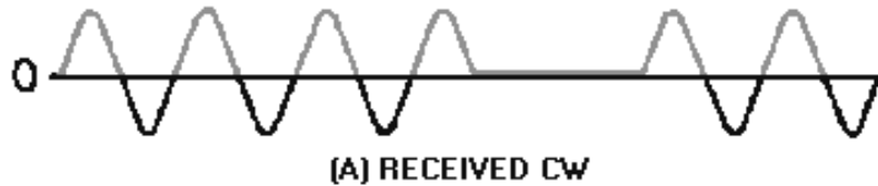
Figure 3-1A.—Cw demodulation. RECEIVED CW.
