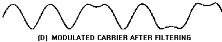
Figure 2-25D.—Phase-shift keying. MODULATED CARRIER AFTER FILTERING.
