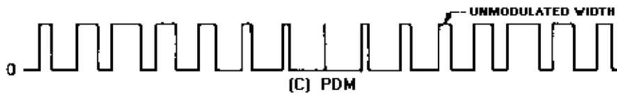
Figure 2-43C.—Pulse-time modulation (ptm). PDM.
