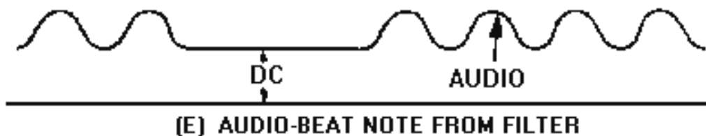
Figure 3-3E.—Heterodyne detection. AUDIO-BEAT NOTE FROM FILTER.
